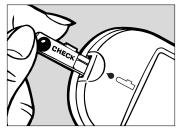
2 Insert the Check Strip fully into the Meter as shown (with tab pointing right). A beep sounds and a full display\* appears. Another beep sounds and the Check Strip test result is displayed. A check mark (✓) shows on the display when the Check Strip test is done.
